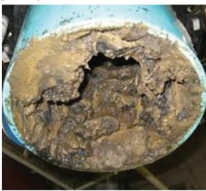
The sewer was almost completely clogged with over 15 tonnes of fat which had reduced the sewer to just five per cent of its normal capacity. The blockage was discovered after local residents complained of being unable to flush their toilets.
